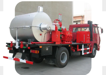
Flushing Units / Sewer Jetting Trucks
